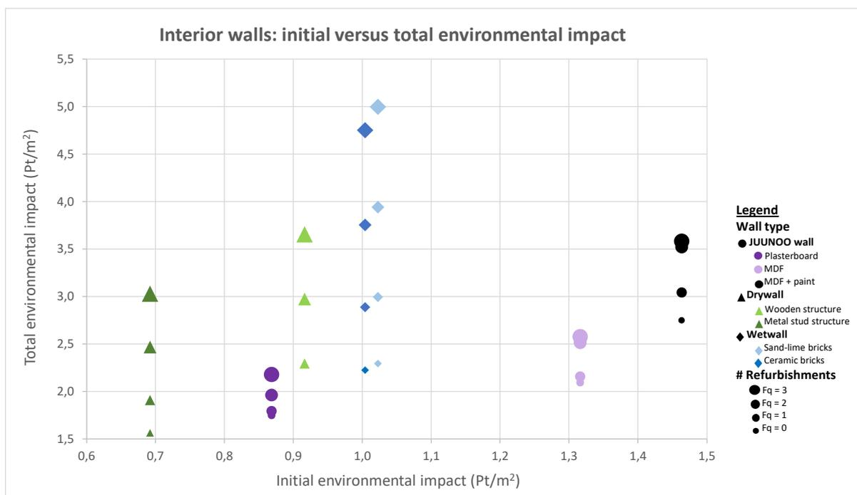
Figure 6.4: Overview of the initial versus the total environmental impact of the different interior walls for four refurbishment frequencies on element level.
