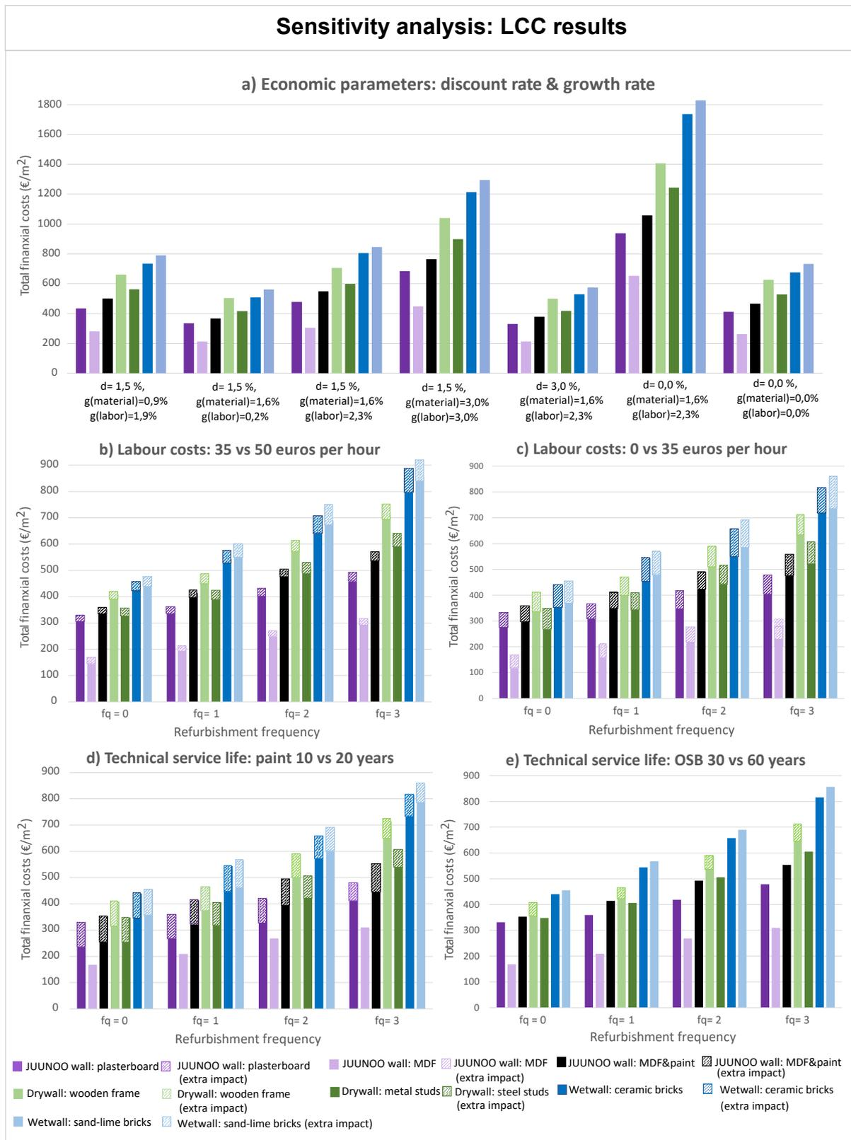
Figure 6.13: Sensitivity analysis on the LCC study, focused on the economic parameters: discount rate and growth rate, labor costs and the chosen technical service life of paint and OSB.
