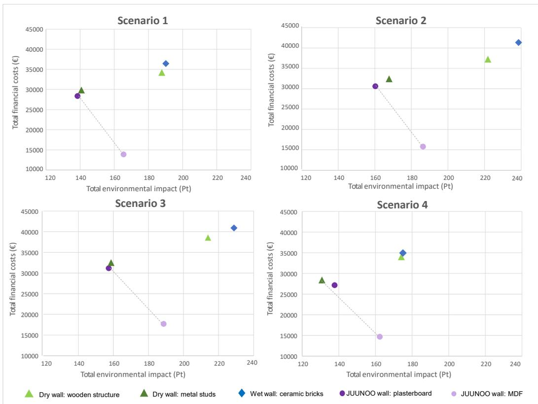
Fig. 4. Comparing the total environmental impact with the total cost of the interior walls using Pareto fronts (dashed lines) for four refurbishment scenarios in the case house in Berchem.
