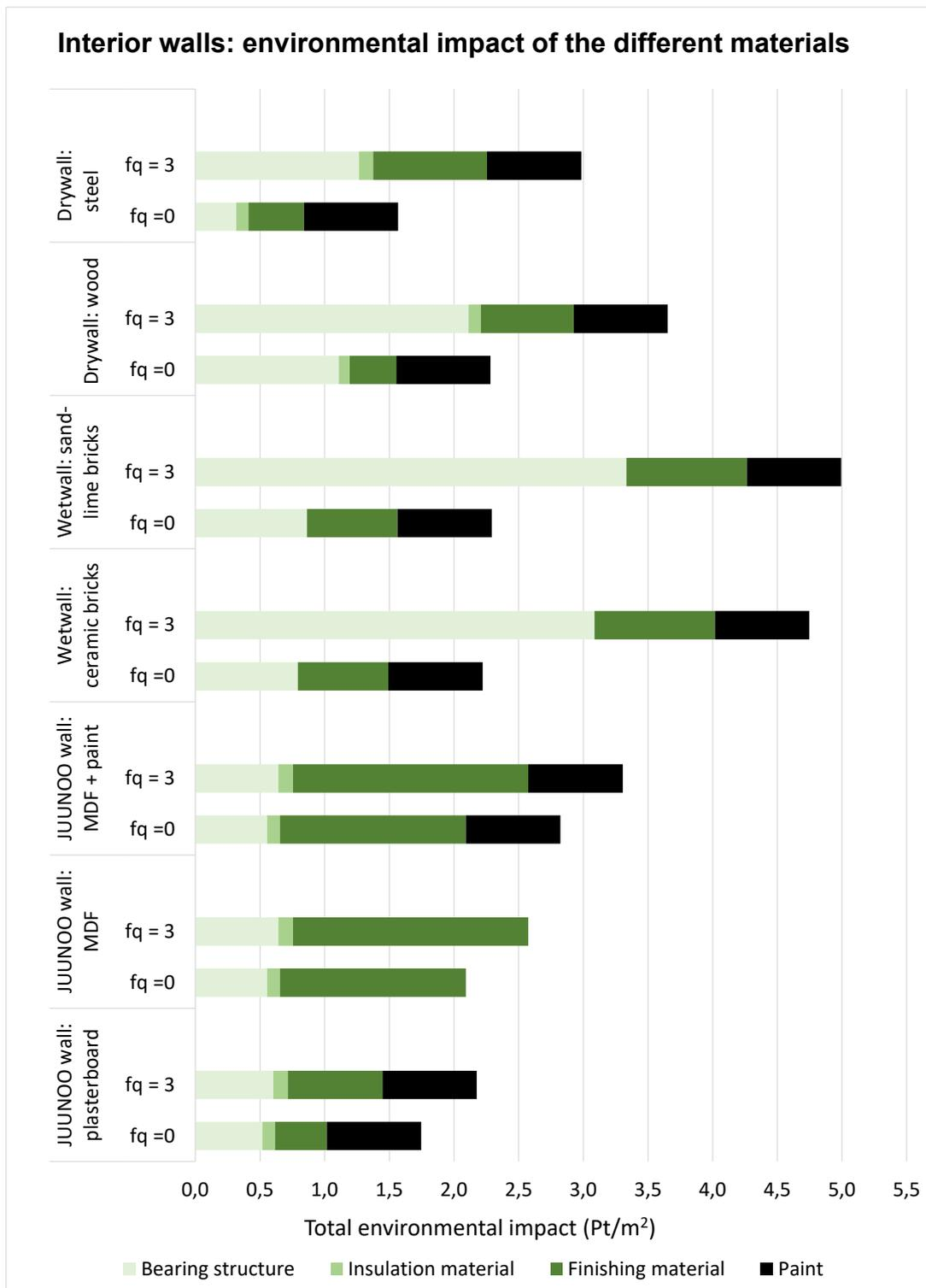
Figure 6.6: Overview of the environmental impact of the different materials for the different interior walls for zero and three refurbishments on element level.
