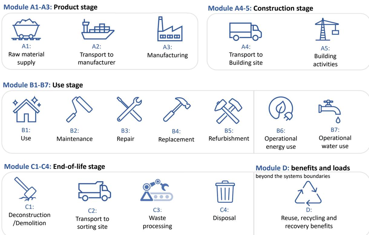
Figure 4.3: Graphical representation of the different stages of the product systems life cycle
