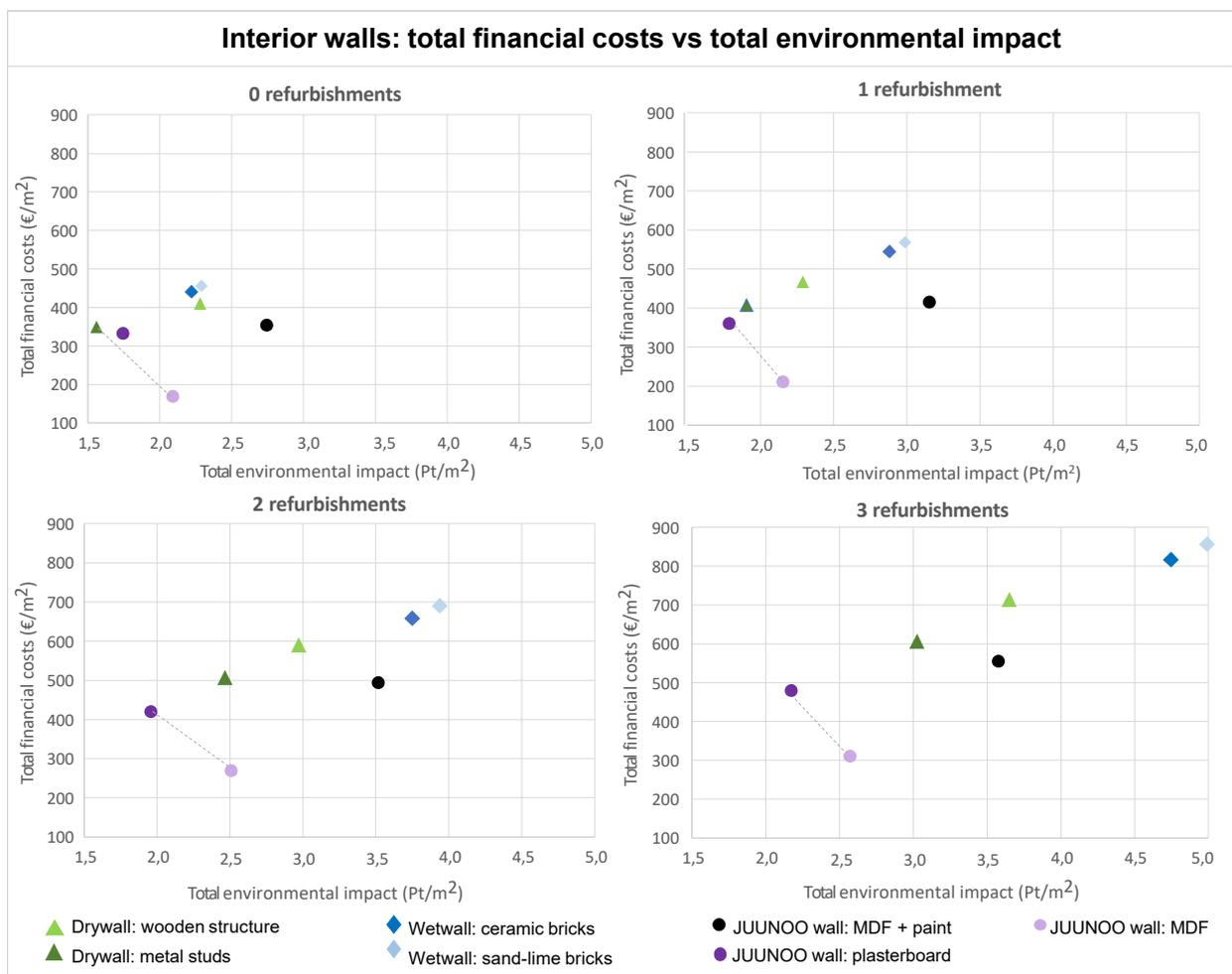
Figure 6.15: Comparing the total environmental impact with the total cost of the interior walls using Pareto fronts (dashed lines) for four refurbishment frequencies on element level.
