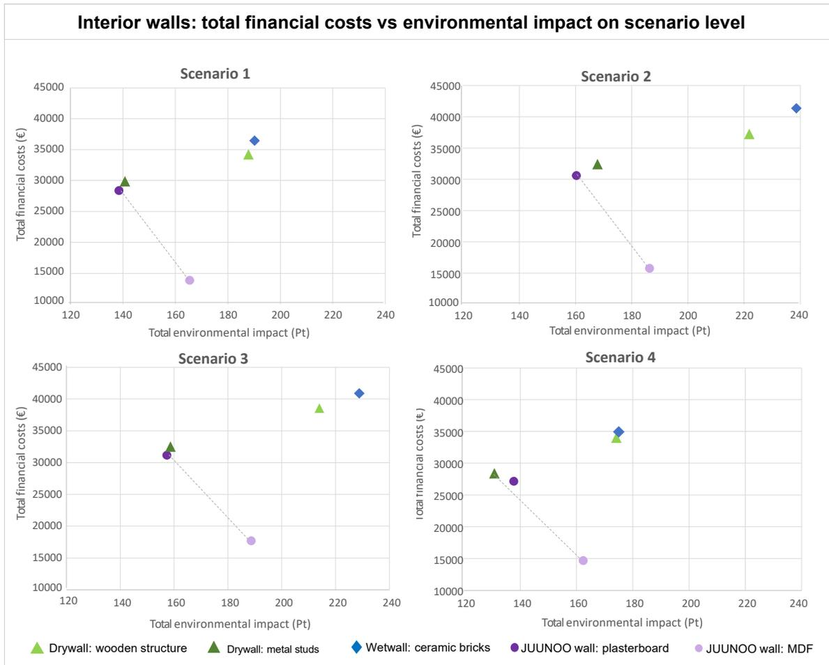
Figure 6.24: Total financial costs vs total environmental impact for the different interior walls for the four scenarios on scenario level.
