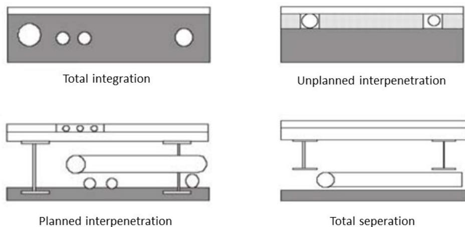
Figure 2.6: The gradation in pace-layering, based on the figures of Durmisevic (2006).
