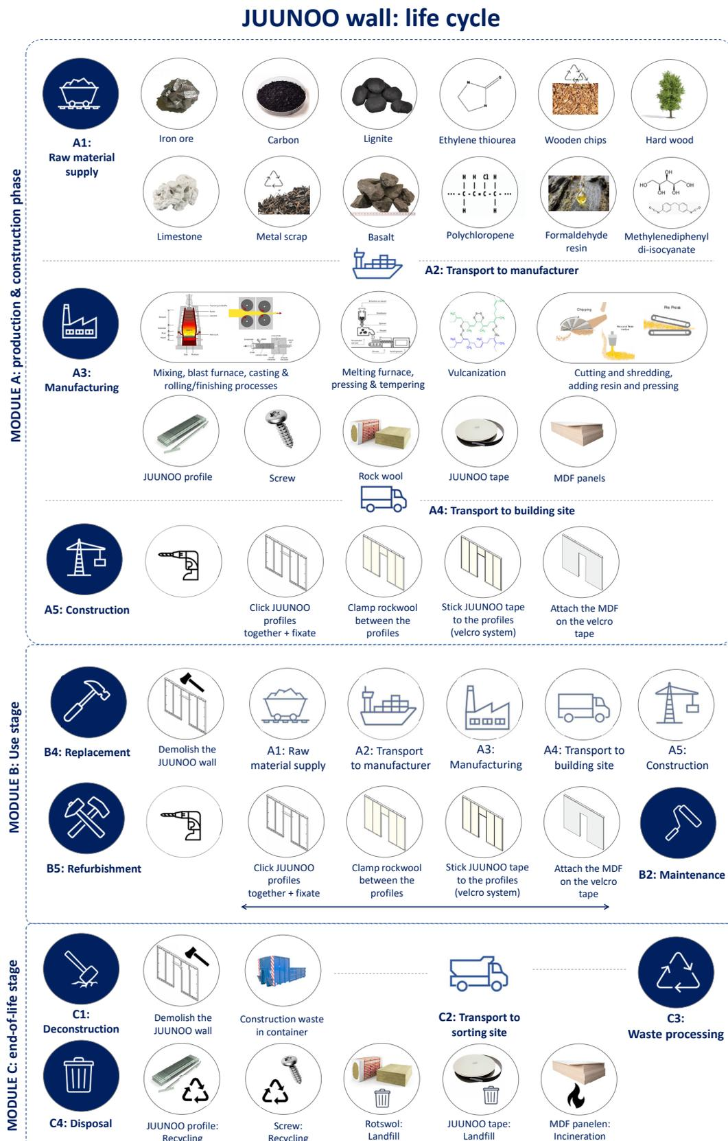
Figure 6.3: The life cycle stages of the reference JUUNOO wall
