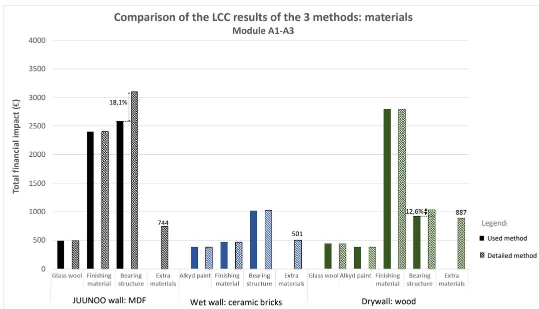
Figure 6.28: Sensitivity analysis on the financial cost of the materials of the wetwall with ceramic bricks, the drywall with wooden frame and the JUUNOO wall with MDF, calculated with the used, expanded and detailed method for scenario 1.
