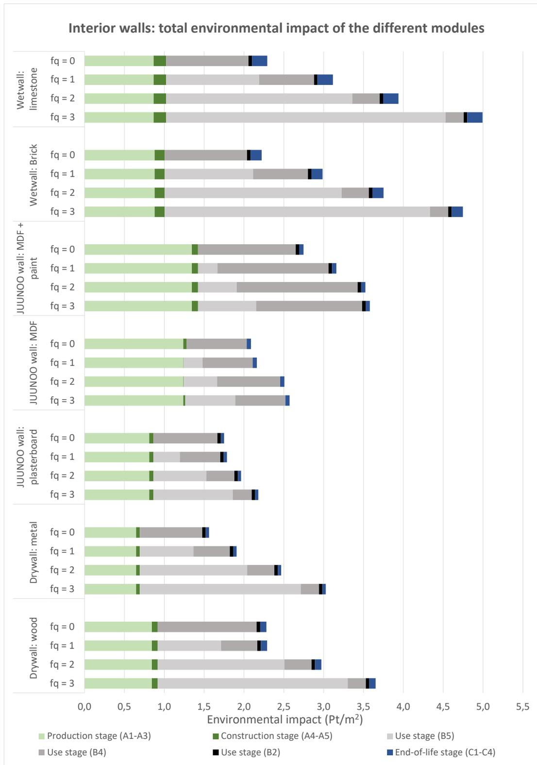
Figure 6.7: Overview of the environmental impact of the different modules of the production, construction, use and end-of-life stage, for the different interior walls for the four refurbishment frequencies on element level.
