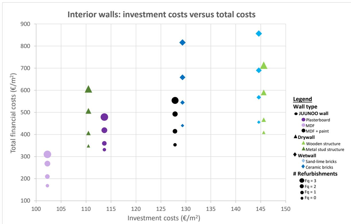
Figure 6.9: Overview of the initial and the total financial costs of the different interior walls for four refurbishment frequencies on element level
