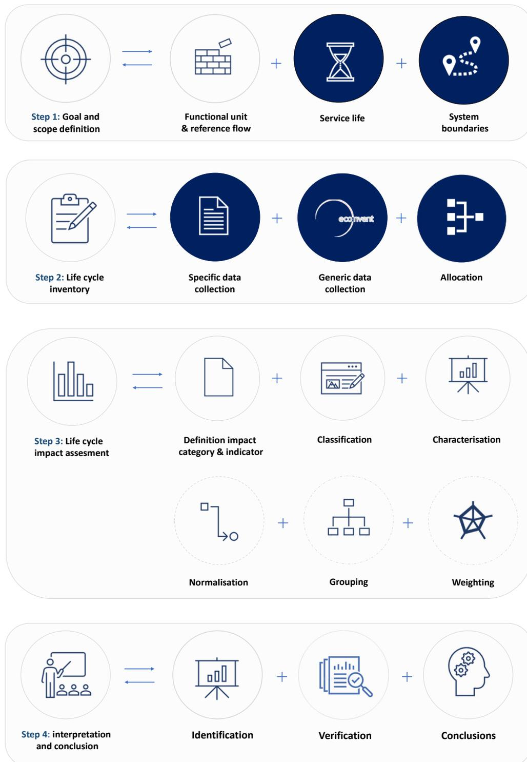
Figure 4.1: The assumptions of the coloured stages: service life, system boundaries, specific and generic data collection, and allocation, need to be modified for the integration of CE in the conventional LCA framework.
