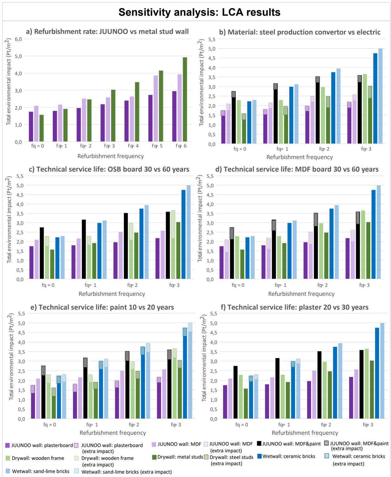
Figure 6.8: Sensitivity analysis on the results of the LCA study, focused on the influence of the refurbishment frequency, the impact of the chosen steel production process, and the influence of the assumed technical service life of the OSB board, MDF, paint and plaster.
