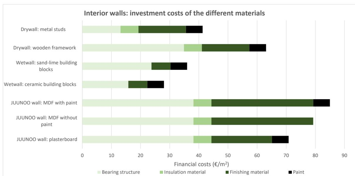
Figure 6.11: Overview of the initial financial costs of the different materials for the different interior walls for zero and three refurbishments on element level.
