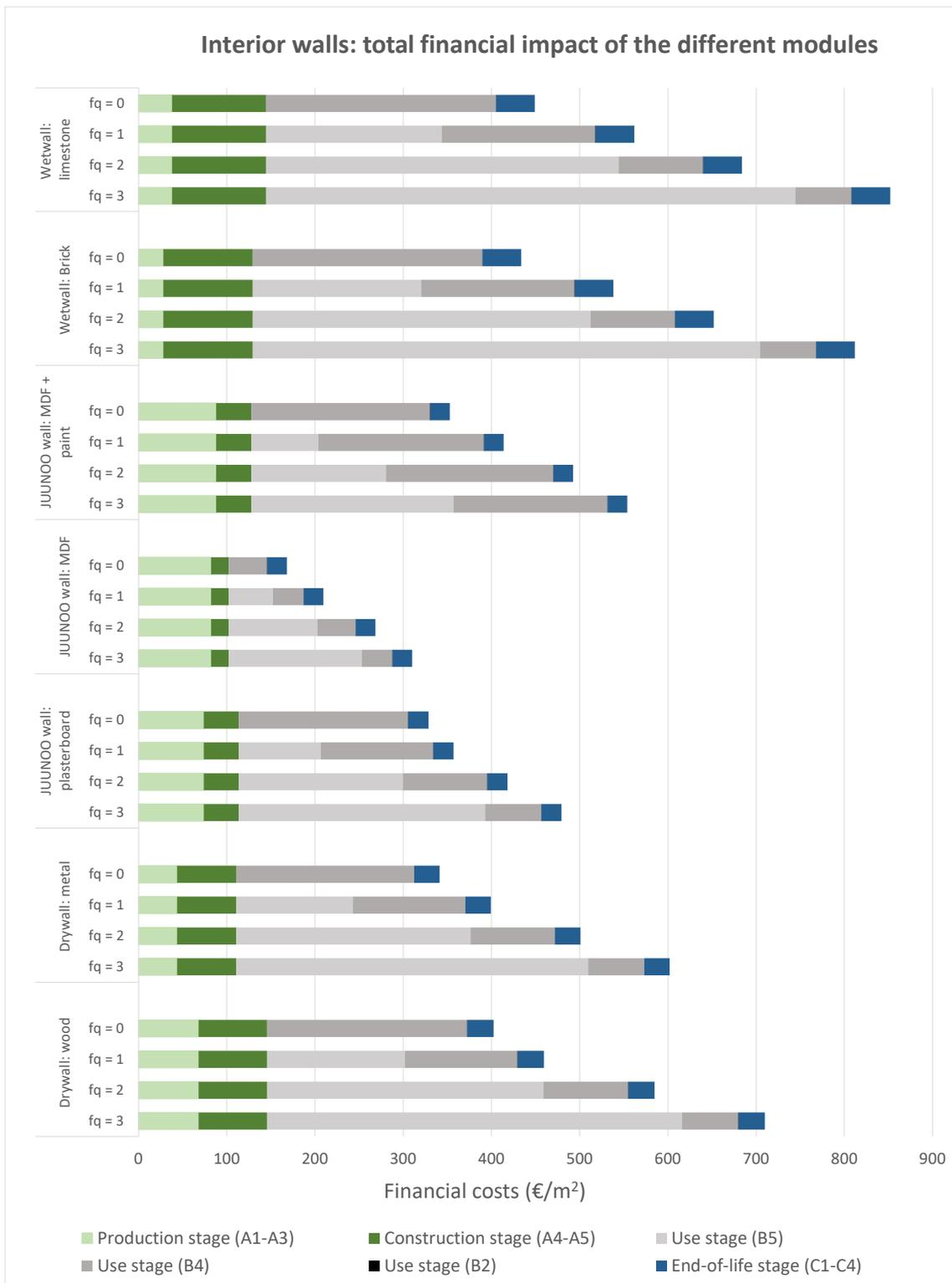
Figure 6.12: Overview of the financial costs of the different modules of the production, construction, use and end-of-life stage, for the different interior walls for the four refurbishment frequencies on element level.
