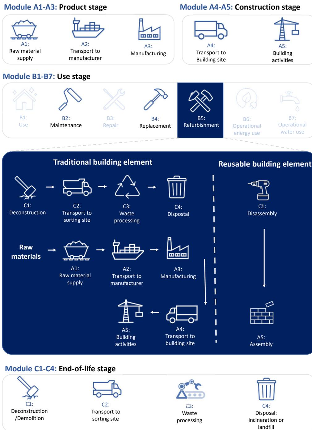
Figure 4.6: The systems life cycle stages of the developed R-LCA framework with the implemented coloured module B5 ‘refurbishment’. The greyed out modules are not implemented in this framework.
