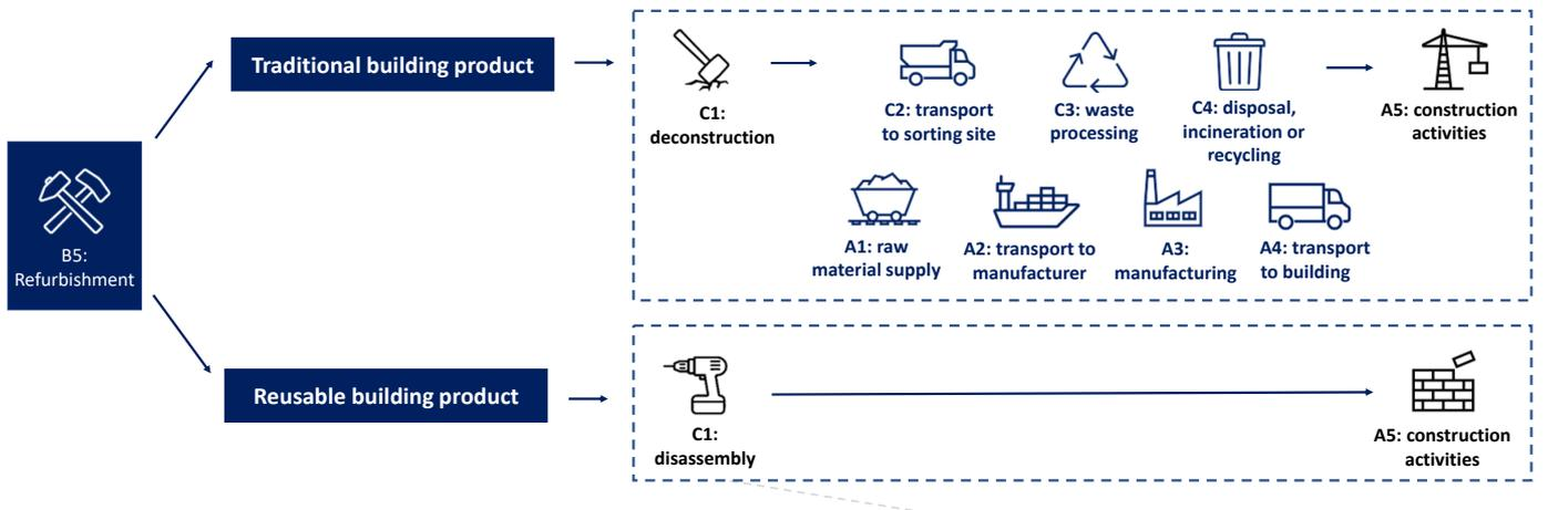
Fig. 1. The implemented module B5 ‘refurbishments’ with the assessed impact modules for reusable and traditional building elements.
