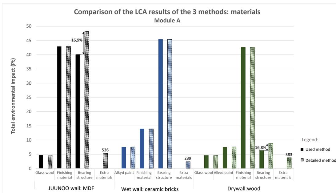
Figure 6.26: Sensitivity analysis on the environmental impact of the materials of the wet-wall with ceramic bricks, the drywall with wooden frame and the JUUNOO wall with MDF, calculated with the used, expanded and detailed method for scenario 1.
