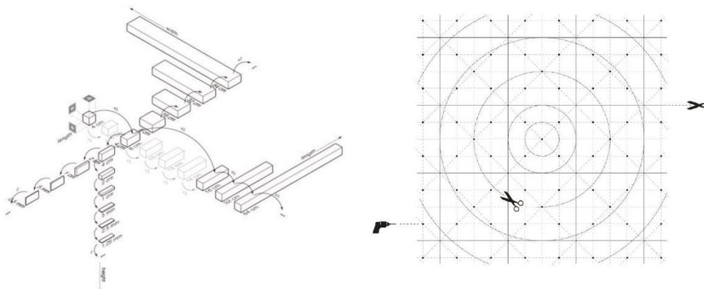
Figure 2.4: The modular sizing system of OpenStructures (2014), based on fractals
