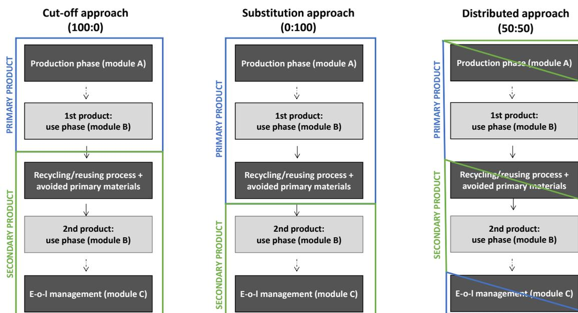
Figure 4.4: Schematic of the three types of allocation methods: the cut-off, the substitution and the distributed approach.
