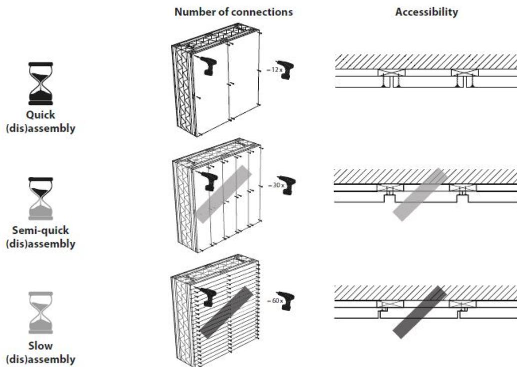
Figure 2.5: The influence of the accessibility and the number of connections on the speed of (dis)assembly, based on Vandenbrouckes leaflets (2017)
