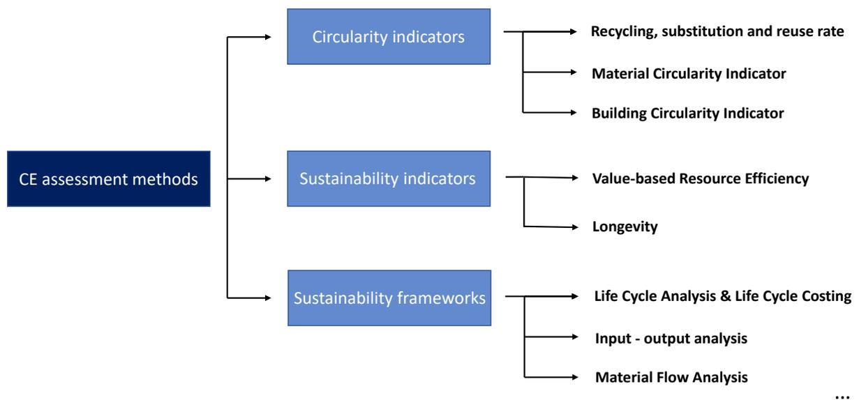
Figure 3.1: Schematic of the current frequent used CE assessment methods in the building industry
