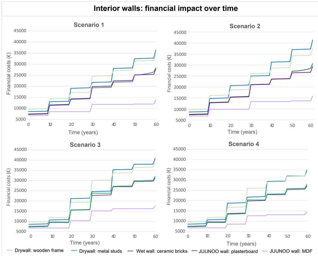
Figure 6.21: Overview of the financial costs over time for the different interior walls for the four scenarios on scenario level.
