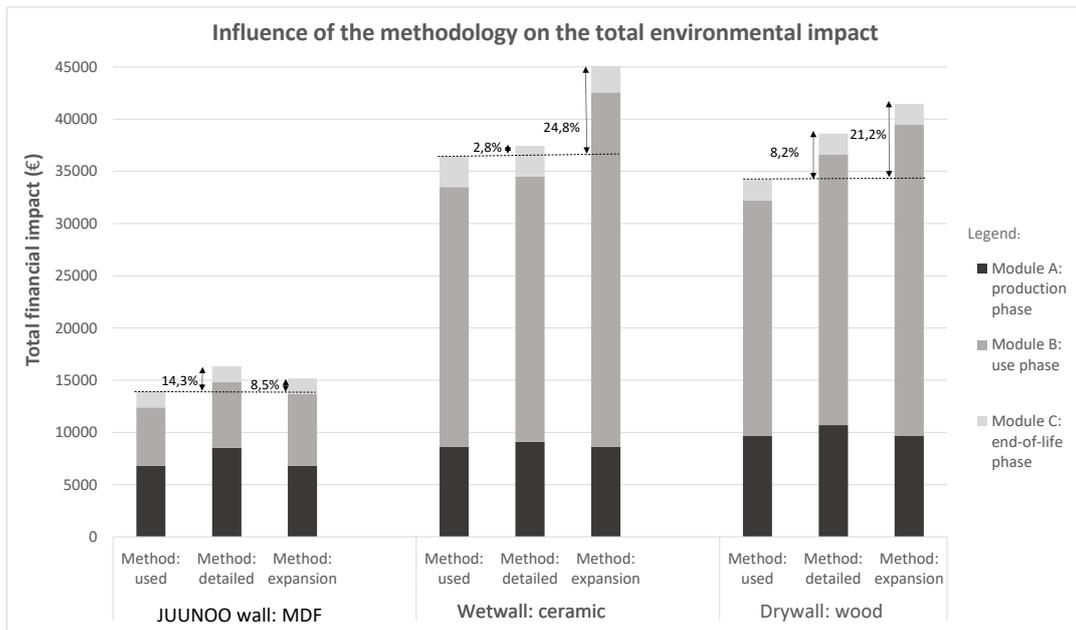
Figure 6.27: Sensitivity analysis on the total financial cost of the wetwall with ceramic bricks, the drywall with wooden frame and the JUUNOO wall with MDF, calculated with the used, expanded and detailed method for scenario 1.
