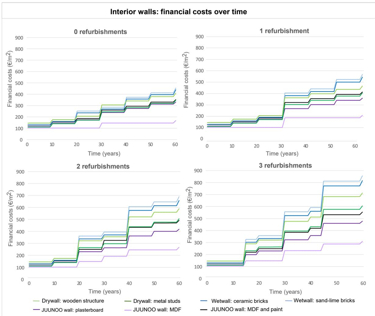
Figure 6.10: Overview of the financial costs over time for the different interior walls for the four refurbishment frequencies on element level.
