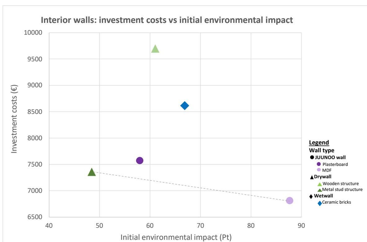
Figure 6.23: Investment costs vs initial environmental impact for the interior walls on scenario level.
