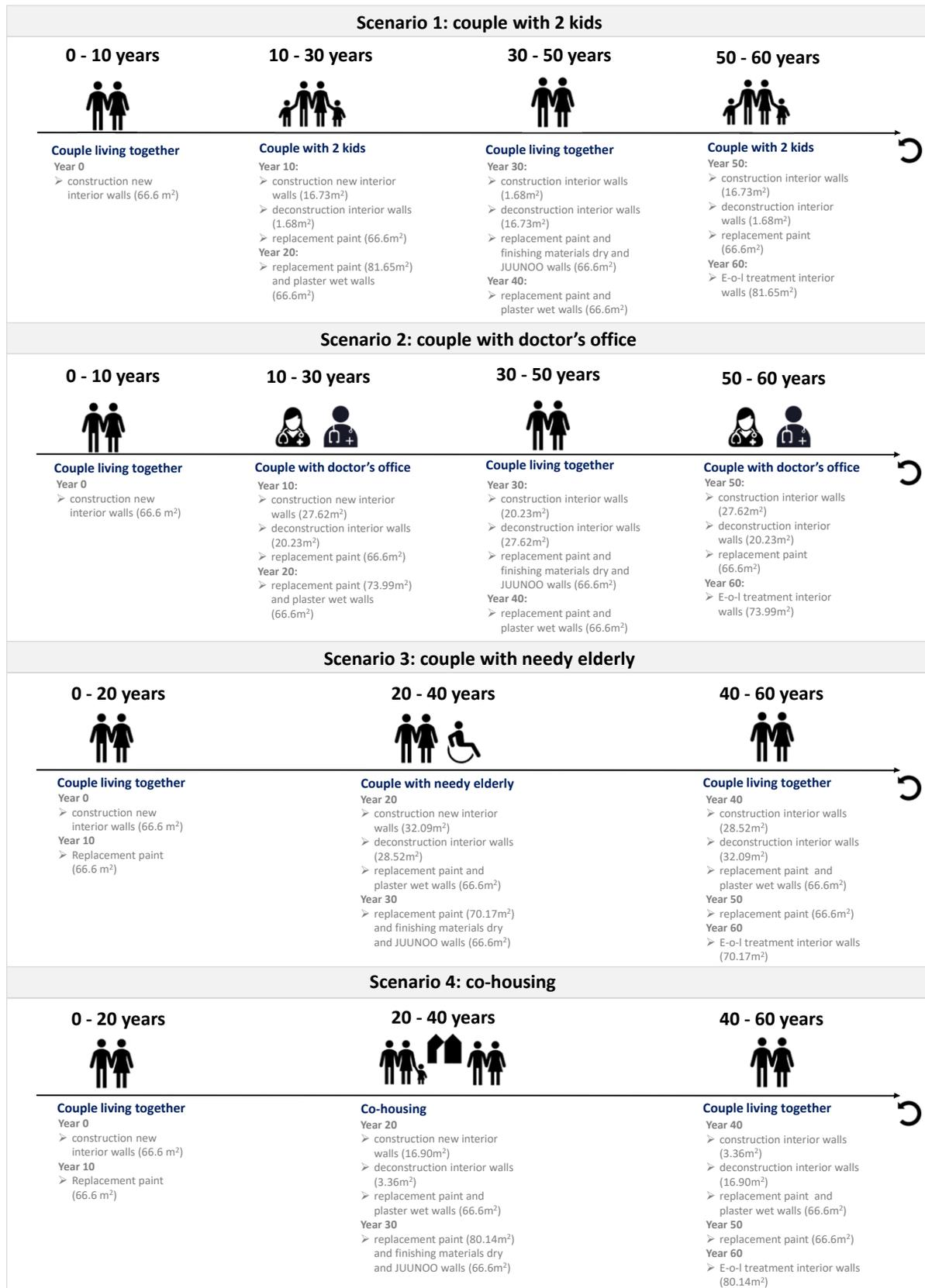
Figure 6.18: Timeline for the four different scenarios, when which material is (de)constructed, replaced or refurbished
