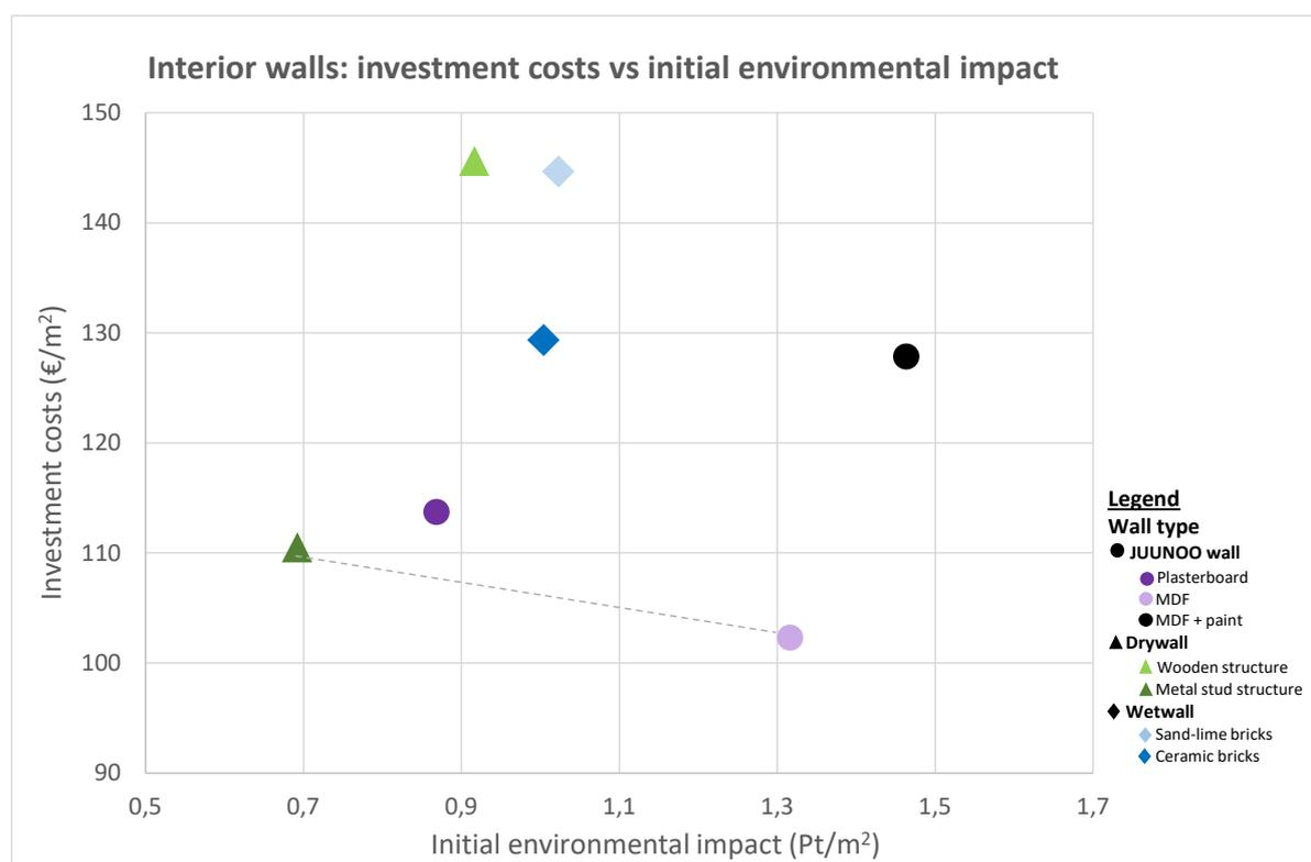
Figure 6.14: Comparing the investment costs with the initial environmental impact of the different interior walls using Pareto fronts (dashed lines) on element level.
