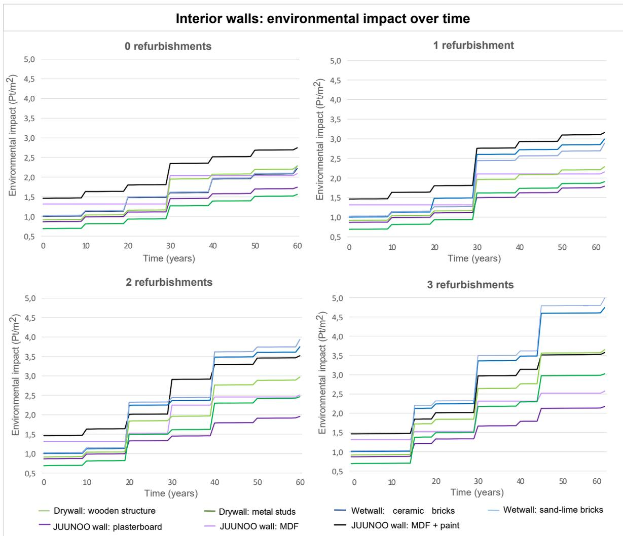
Figure 6.5: Overview of the environmental impact over time for the different interior walls for the four refurbishment frequencies on element level.
