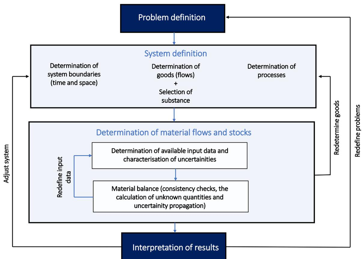
Figure 3.3: The four steps of the MFA methodology, based on the theory of Brunner and Rechberger (2004).
