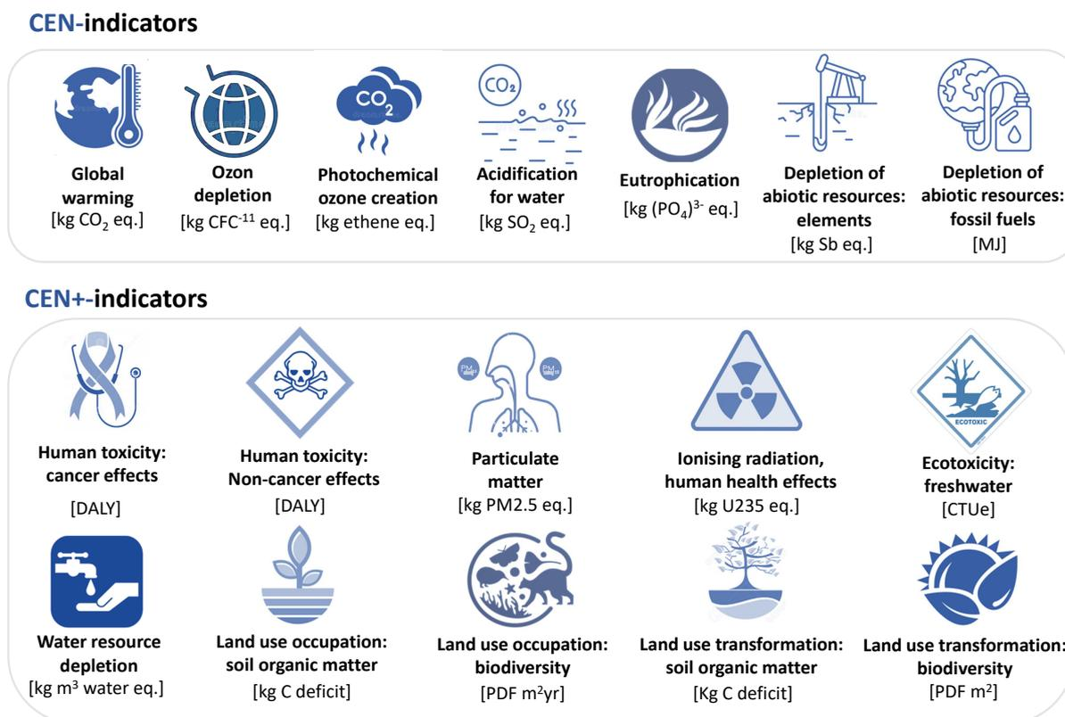
Figure 4.5: Scheme of the CEN and CEN+ indicators, proposed in the NBN EN 15804, with their basic unit.
