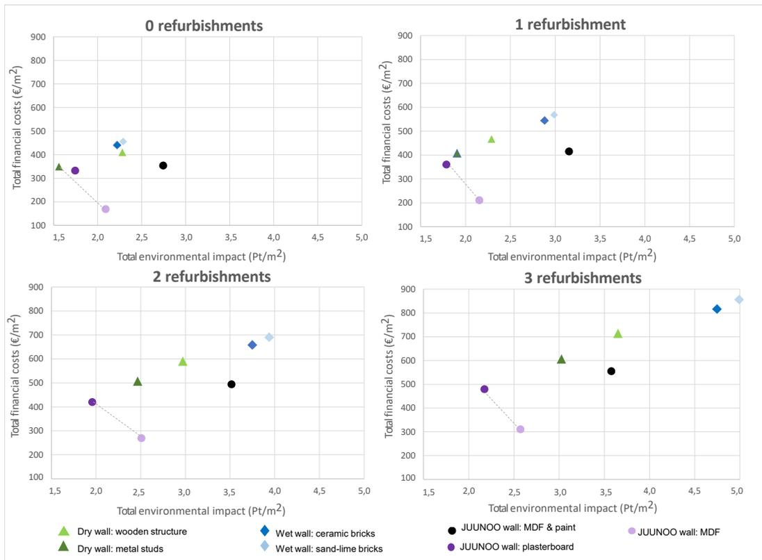
Fig. 3. Comparing the total environmental impact with the total cost of the interior walls using Pareto fronts (dashed lines) for four refurbishment frequencies on element level.
