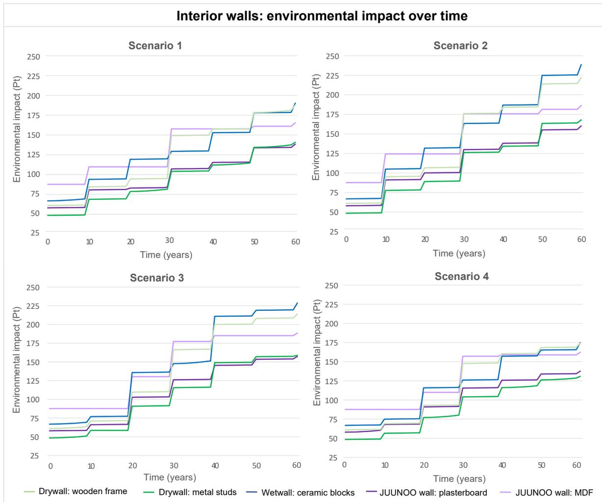
Figure 6.19: Overview of the environmental impact over time for the different interior walls for the four scenarios on scenario level.
